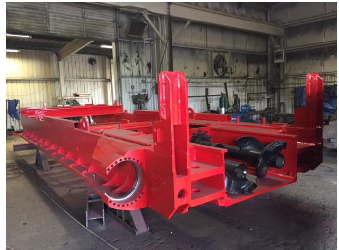
Highwall Miner Frame in Manufacture
