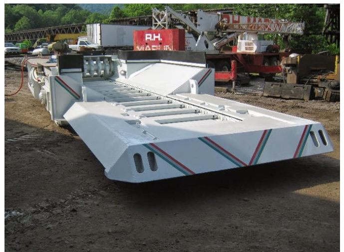
Auxier Welding Feeder Breaker
